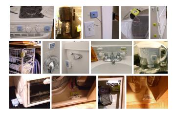
Fig. 2. Examples of some of the 77 sensors that were installed in the home of the first subject. The sensors and data collection boards were literally taped to objects and surfaces for the duration of the data collection period.
