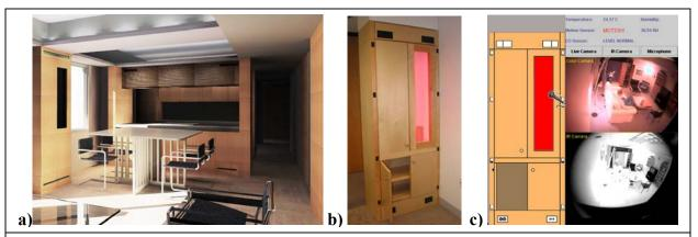
**Figure 2:** (a) A rendering of the living room of the PlaceLab, showing one cabinet on the left. (b) A prototype of that cabinet. Each cabinet has sensors for color video, infrared video, temperature, position, motion, doors, audio, and air quality. This cabinet also has audio output, 24-bit color output (red nook), and infrared floodlights. (c) A display showing the state of the doors, lighting, environmental sensors, and the two video streams from the prototype cabinet, updated in real time.
